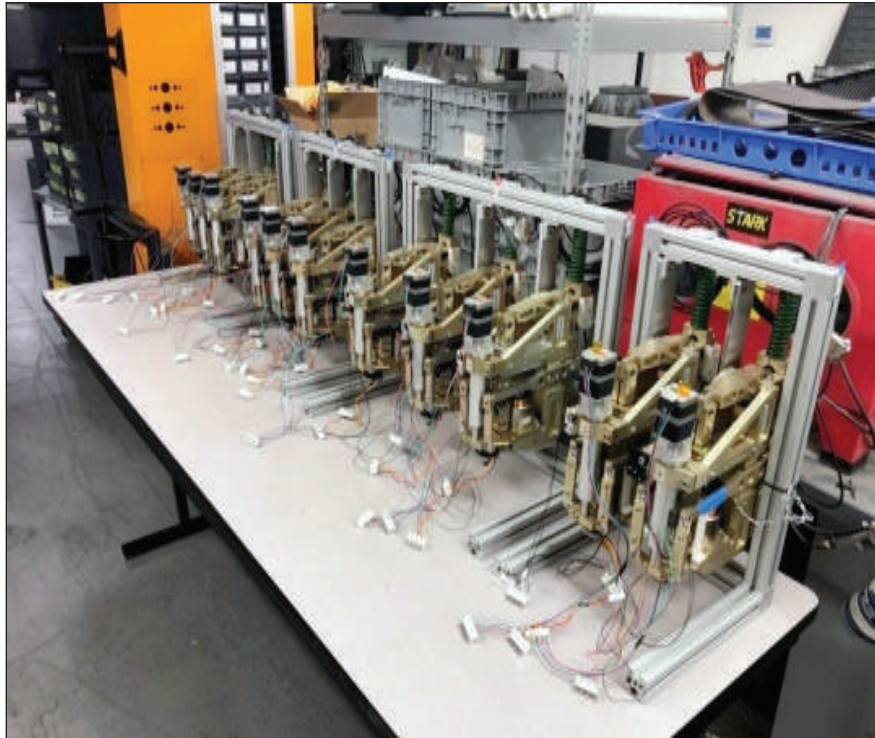
Fig. 6: Actuators made in India undergoing life-cycle tests
