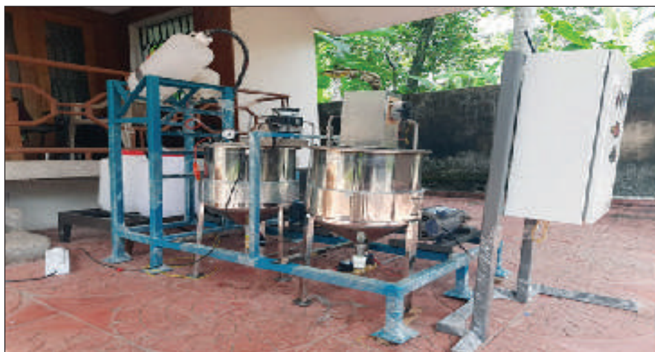
Fig: Prototype developed for Biocatalytic system for the re-purpose of used cooking oil by PC SCTIMST-TIMED, (SreeChitraTirunal Institute, Trivendrum)
