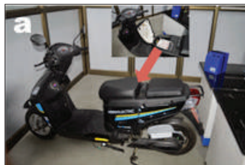
E-scooter with NMC/graphite module of 48V, 1 kWh
