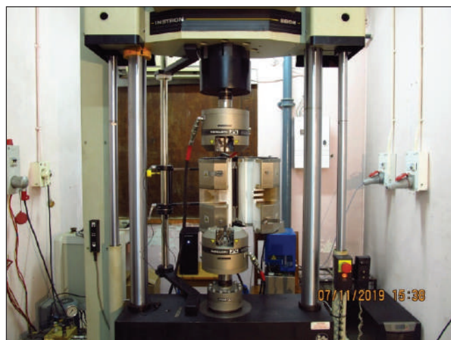
Electric Universal Testing Machine with Furnace acquired under DST FIST at Department of Metallurgical and Material Engineering, Jadavpur University, Kolkata
