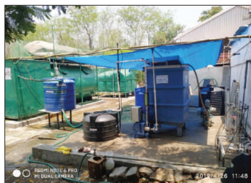
Aerobic Moving Bed Bioreactor (MBBR) + side stream NF integrated with anaerobic gas lift reactor (AGR)
