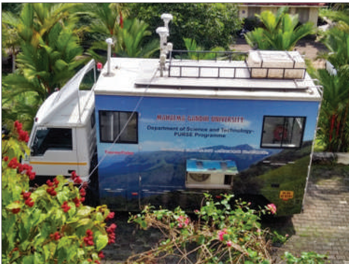
Fig. Mobile Ambient Air Pollution Monitoring System established out of DST PURSE at Mahatma Gandhi University, Kottayam Kerala
