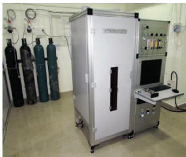
Four mirror optical floating zone crystal growth system acquired under DST FIST at Anna University Chennai
